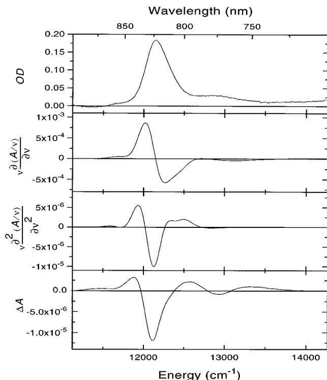
**Figure 2.** From top to bottom we show the 77 K absorption spectrum and first- and second-derivative spectra and the Stark spectrum of a preparation of B820. The Stark spectrum was measured at  $\chi = 54.7^\circ$  and the electric field strength  $F = 1.0 \times 10^5 \text{ V cm}^{-1}$ . The derivative spectra were calculated from a fit to the absorption spectrum.
