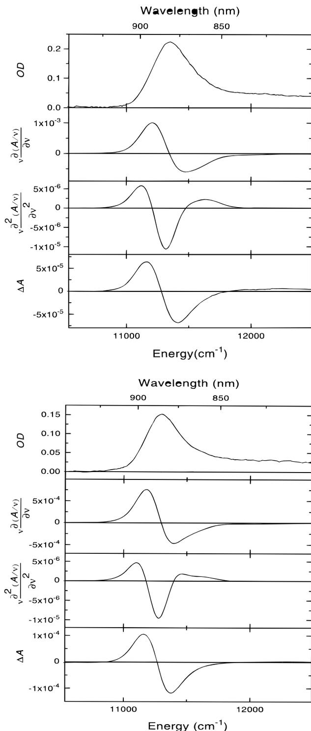
**Figure 4.** The 77 K absorbance-, first derivative-, second derivative-, and Stark spectra measured at  $\chi = 54.7^\circ$  and at a field strength of  $F = 1.0 \times 10^5 \text{ V cm}^{-1}$  of (A) M2192 and (B) reconstituted B873 complexes.
