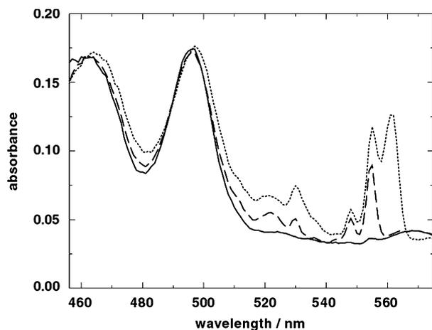
**Fig. 5.** Absorbance spectra of the cyt *b<sub>6</sub>f* complex from the CrtO-less mutant at 4 K. The spectra were recorded in the presence of 100  $\mu$ M ferricyanide (solid line), 20 mM ascorbate (dashed line), or after addition of a few grains of dithionite (dotted line). The carotenoid absorption bands peaking near 496 and 462 nm shift to the red upon reduction of cyt *b<sub>6</sub>*.
