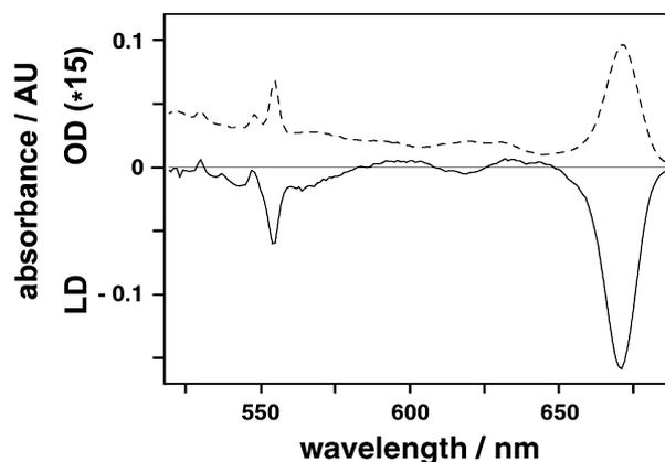
**Fig. 3.** Comparison of absorbance and LD spectrum. The absorbance spectrum in the chlorophyll region (upper half, dashed line) and the LD spectrum (lower half, solid line) of the ascorbate-reduced, isolated cytochrome *b<sub>6</sub>f* complex from the Crto-less mutant at 77 K are compared. The LD spectrum was recorded using cytochrome *b<sub>6</sub>f* complexes oriented in a two-dimensionally squeezed gelatin gel. The values on the y-axis represent the absolute absorbance and LD values.
