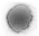
at Lund University predicted that optimized HHG produces EUV with significant spatio-temporal coupling (STC) [171]. In short, this implies that the electric field of the lightwave cannot be expressed as the product of a spatial wave profile and a temporal wave profile. STC can appear in many forms, but the predicted STC [171] is very similar to the chromatic aberration produced by chromatic lenses in the visible domain.
