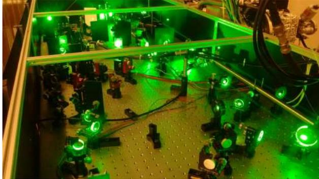
Figure 2.8: Photo of the NOPCPA amplifier in action. The left side of the image shows the first two amplification stages of the NOPCPA, the bright spot in the center shows the final amplification stage and the right part shows the relay imaging system of the pump beam for the final amplification stage.
